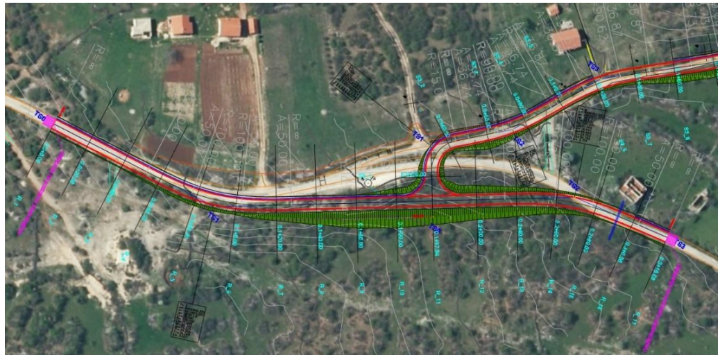
Figure 3-30: Design situation of the section SR3, relocation of the existing road and newly designed T-interchange
