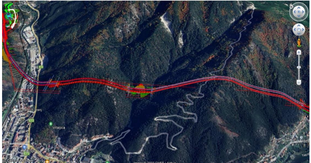
Figure 3-2: Viaduct 3 over Tresanica, Tunnel 1 and Tunnel 2 (source: Google Earth)
