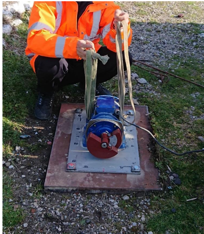
Figure 12-3: 250 kg Vibration generator
