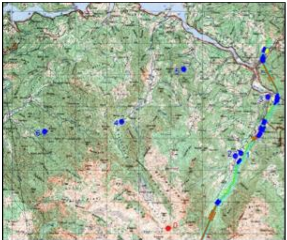
Figure 7-21: Place of dye injection at Jezero (0) and monitoring locations (1- 4)
